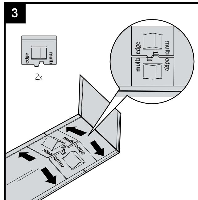
Push the connector strips underneath the top and bottom edge of the profile. Do this at the seam where the profile transitions to the corner piece. Make sure that the connector strips fit together.
