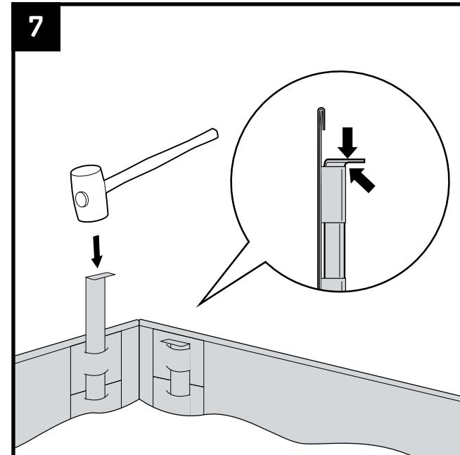
Gently tap all the fixing stakes into the soil with a hammer until the top comes into contact with the connector strips. Close the seams at the ends of the profiles and corner pieces by pressing the ends together and then gently push the fixing stake into the soil.
