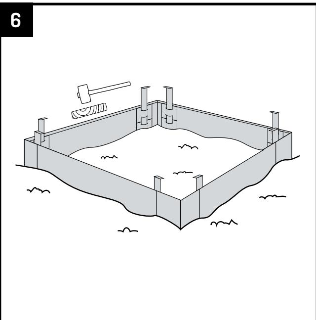
Place the planter into the channel. Gently tap down the profiles to the desired height. Use a wooden block to avoid damaging the profiles. For stability, leave no more than 10 cm of the profile protruding above the surface of the soil.
