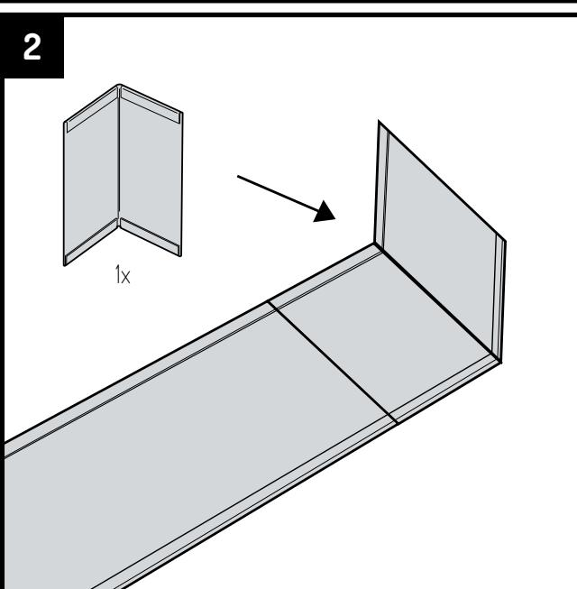
The profiles are connected to each other by anchoring the corner pieces with connector strips and fixings stakes. Therefore, start by attaching all the corner pieces to the profiles. Place the corner piece against the profile.
