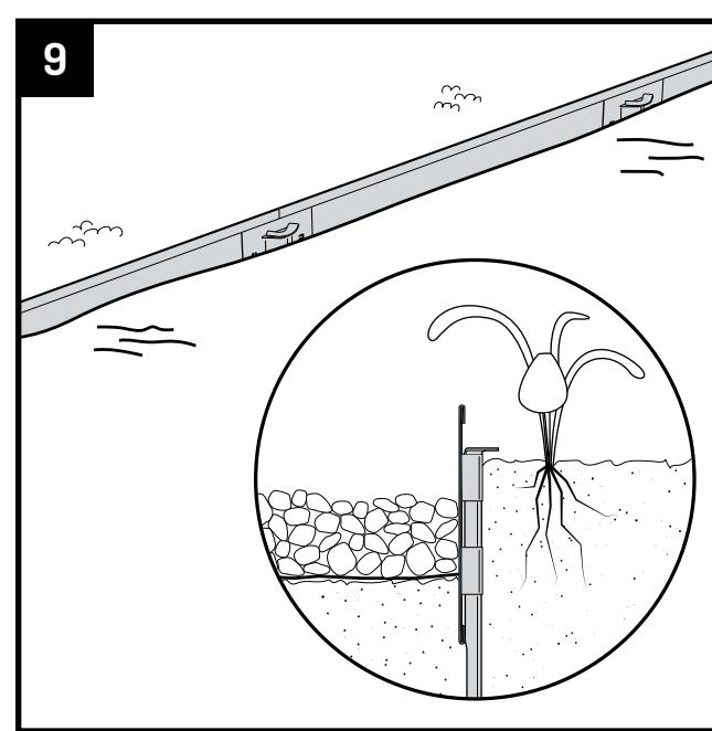
Backfill the channel with soil, sand or another material. Then lay grass, gravel or another type of ground cover up to the edging.
