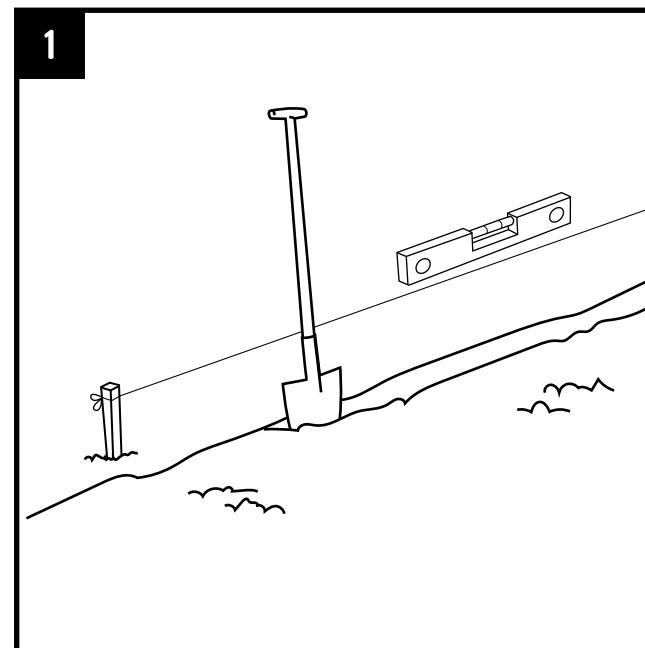
Mark out the line along which the Multi-Edge ADVANCE is to be installed with twine and pegs. Dig a channel at least 10 cm deep along that line.
